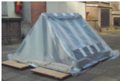
Figure 12. Solar Tent placed on blocks with outer tent clipped to floorboard.
