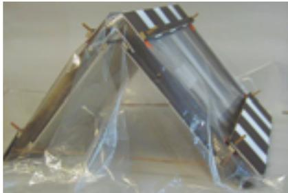
Figure 11. Outer cross supports with extra surface
